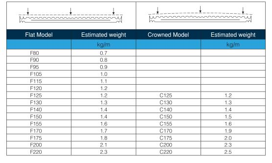
The values shown are nominal widths corresponding to the width of the rail foot. C200 is a crowned pad suitable for the DIN rail A100. RailLok™ *double-crown* pad is supplied in rolls with standard lengths of 12 meters, tolerances on length is ± 50 mm.
